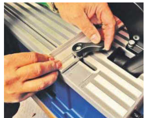
Common timber dimensions are marked to help set the fence
